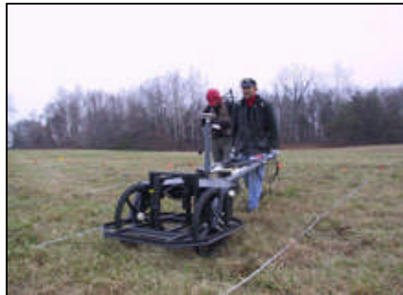
Figure 1: Mapping with a cart-mounted Dynamic NanoTEM (DNT) system.
