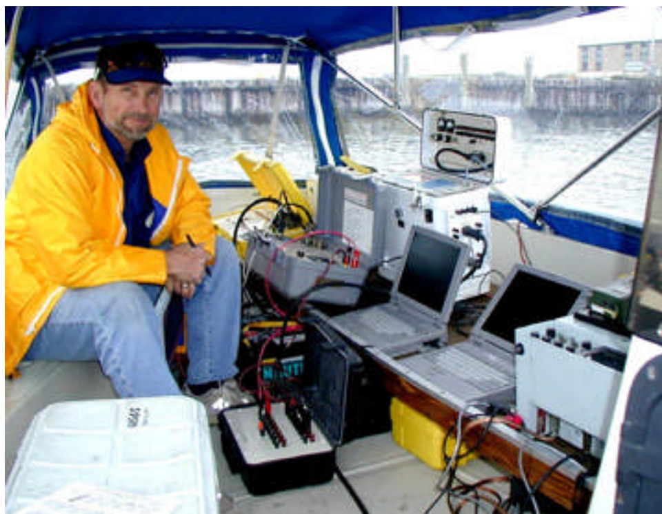
Figure 3. Instrument setup inside powerboat. To left: resistivity control and data acquisition system, with Donald Snyder. To right: GPS navigation recording equipment.
