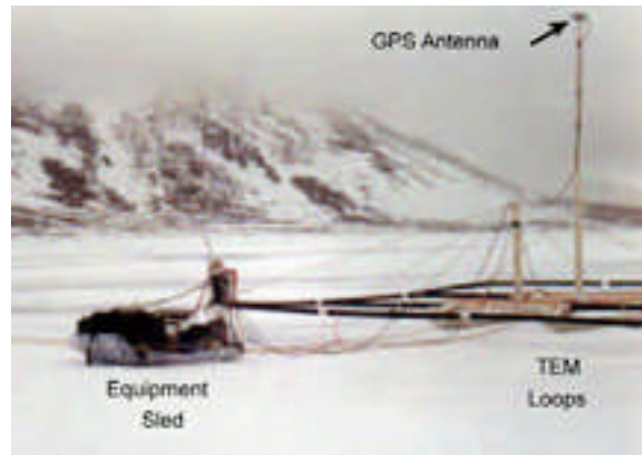
Figure 2: A sled mounted TEM system was towed across thick lake ice in May 2000. A real-time differential GPS system recorded accurate positions. TEM transients were recorded at 26 times spaced logarithmically between 7 and 570 usec.
